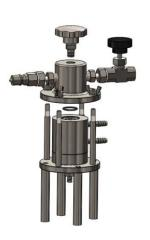
(1) Assemble the middle O-ring (9) into the groove at the bottom of the extruder top (6). (2) Mount the extruder top (6) and tighten it in order with gaskets (11) and wing nuts (12). (3) Tighten the inlet cap screw (5) by screwing it
