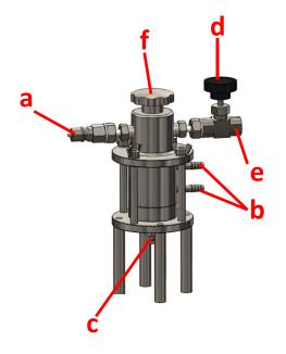
a: connected to the female of the provided high-pressure nitrogen tubing 13
