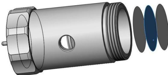
Carefully place the sintered disc, membrane, sintered dish on the assembly components of O-ring (4) and O-ring support (3) in step 2. Note: The Nanopore membrane must be flat and wet without any wrinkle or bubble.
