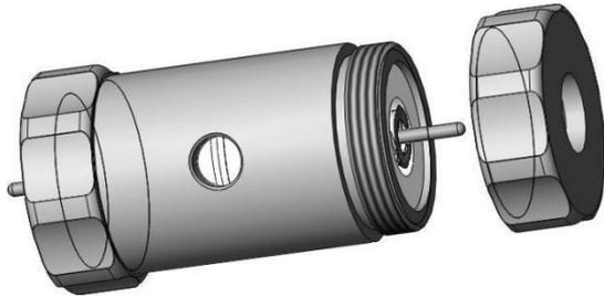
Connect another container nut (1) to the housing (2), and tighten two container nuts (1) on the housing (2) firmly.
